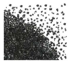
(Rockwell Hardness: 68HRC) Hardness 6 - 7 Moh scale Specific gravity (ASTM C128-15) 3 Average bulk density ≈ 1,84 g/cm<sup>3</sup> (ASTM D7481-09) (NIOSH 7602) Crystalline silica < 0.15% Conductivity <150 µS/cm (ASTM D4940-98-15e1) pH (1% Solution) 6.13 (ASTM E70-07(15)) Moisture content <0.05% (ASTM C566-13) Oil content (ASTM D7393-16) None
